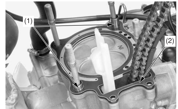
(1) dowel pins (2) cylinder head gasket
