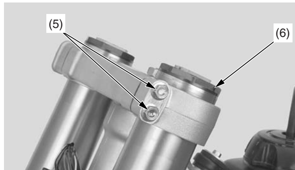
(5) upper pinch bolts (6) fork damper
