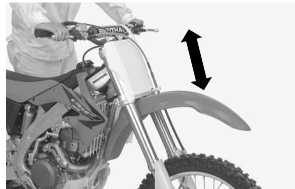
27. Tighten the left fork pinch bolts (28) alternately first. While keeping the forks parallel, alternately tighten the right fork pinch bolts (28) to the specified torque:
