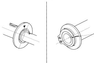
For added security, you may choose to safety wire the hand grips to the handlebar and throttle to prevent the possibility of them loosening. Position the twisted wire ends away from your palms and be sure to bend the wire ends well into the grip rubber so they will not snag your glove.
