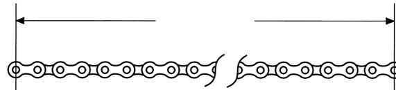
MEASURE A SPAN OF 17 PINS (16 PITCHES)
