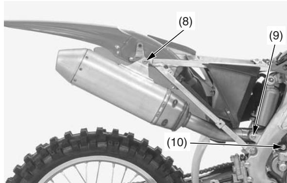
(8) muffler B bolt/washer (10) muffler clamp bolt
