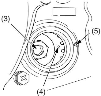
(3) primary drive gear lock bolt (5) index mark
