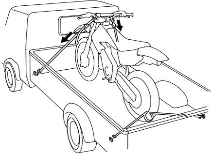
To secure your CRF, brace the front wheel against the front of the truck bed or trailer rail. Attach the lower ends of two straps to the tie-down hooks on your vehicle. Attach the upper ends of the straps to the handlebar (one on the right side, the other on the left), close to the fork.
