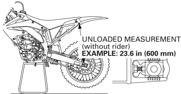
3. Measure the *loaded with rider* dimension. Remove the workstand. With two helpers available, sit as far forward as possible on your CRF's seat, wearing your riding apparel. Ask one helper to steady your CRF perfectly upright so you can put both feet on the pegs. Bounce your weight on the seat a couple of times to help the suspension overcome any situation and settle to a good reference point.
