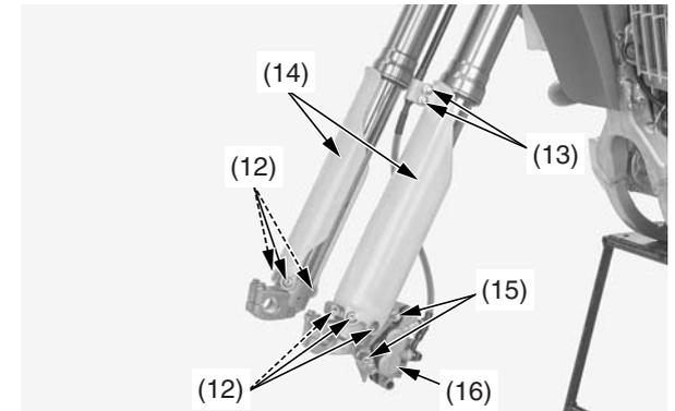
(12) fork protector bolts (15) brake caliper bolts
