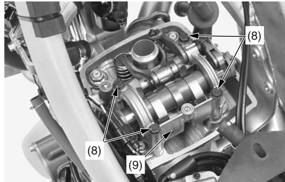
(8) camshaft holder assembly bolts
