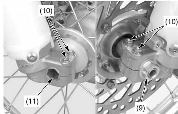
(9) axle nut (11) front axle shaft
