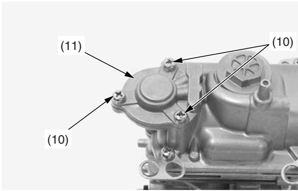
(10) accelerator pump cover screws
