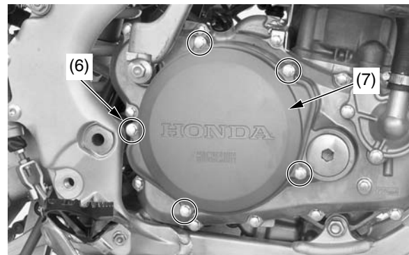
(6) clutch cover bolts (7) clutch cover
