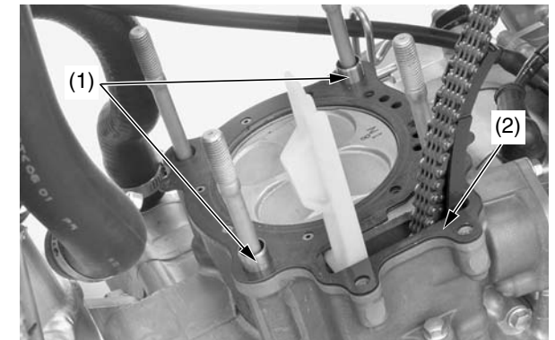
(1) dowel pins (2) cylinder head gasket
