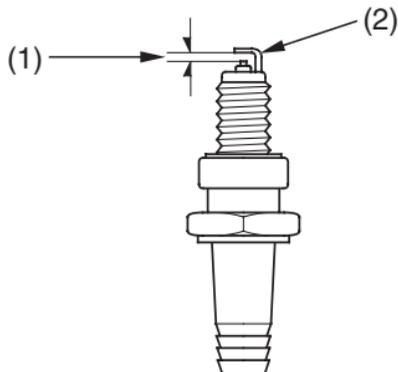
(1) spark plug gap    (2) side electrode
