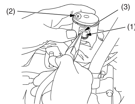
(1) piston pin (2) "IN" mark
