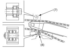
(7) upper drive chain roller (8) lower drive chain roller
