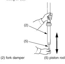
7. Extend the fork damper piston rod to maximum. Adjust the oil level of the fork damper (2) as shown.
