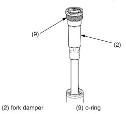
7. Tighten the fork damper using the special tool, to the specified torque: 25 lb·ft (34 N·m, 3.5 kgf·m)
