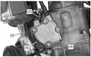
(2) bolts (3) clamp (4) RC cover (5) gasket 4. Loosen the lock nuts (6) and disconnect the RC valve control cables (7) from the RC valve pulley (8).
