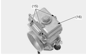
(15) float chamber screws (16) float chamber
