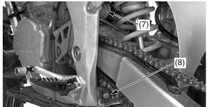
(7) upper drive chain roller (8) lower drive chain roller
