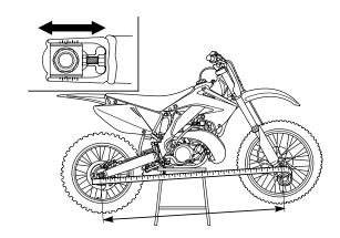
You can "adjust" the power delivery of the standard engine to suit track conditions by changing gearing. This allows you to utilize a different portion of the engine's power range at a given throttle setting. New gearing may provide the change you are looking for without the need to consider further modifications.
