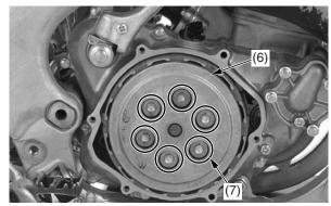
(6) clutch pressure plate (7) clutch spring bolts
