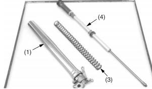
(1) outer tube/slider(3) fork spring
