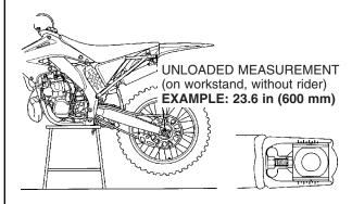
3. Measure the *loaded with rider* dimension. Remove the workstand. With two helpers available, sit as far forward as possible on your CR's seat, wearing your riding apparel. Ask one helper to steady your CR perfectly upright so you can put both feet on the pegs. Bounce your weight on the seat a couple of times to help the suspension overcome any stiction and settle to a good reference point.
