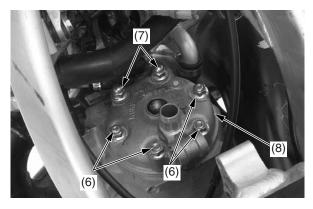
(6) cylinder head nuts A(7) cylinder head nuts B/washers
