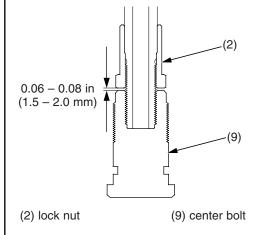
9. Tighten the lock nut (2) to the fork center bolt (9) closely by hand. Tighten the lock nut to the specified torque:
