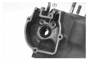
(1) valve shaft oil seal
