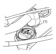
(1) compression damping adjuster screw
