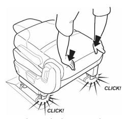
5. Raise the seat-back to an upright position, then rock the seat back and forth, trying to tilt it forward, and make sure both the inner and outer latches are locked in position.
