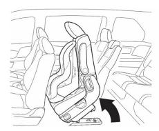
American Honda does not recommend using this method to access the third row seats. When the second row outer seat is tipped forward, the seat may slide into the area between the standard and wide positions that prevents the seats from latching. Therefore, using this method of access increases the risk of having an unsecured second row outer seat.
