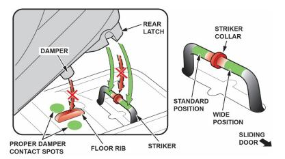
Check that the seat is latched by rocking the seat back and forth, trying to tilt it forward, and make sure both the inner and outer latches are locked and the front seat hooks are under the front latches.
