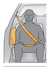
Side airbags are designed to help protect a front occupant's chest.
