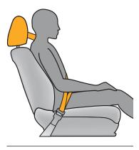
Adjusting a head restraint so the center is level with the back of the occupant's head (or as high as possible for taller people) can help reduce injuries during a rear impact.
