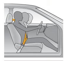
In a moderate-to-severe frontal crash, the seat belts lock to restrain the occupants, and tensioners tighten the front seat belts.
