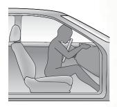
Without a seat belt or an airbag, the occupant will continue forward at 30 mph until they strike the interior of the car with enough force to cause serious injuries.
