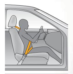
If the driver's seat position sensor detects a driver is closer to the steering wheel than recommended, the airbag will inflate with the least force possible.
