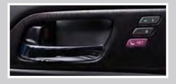
4. Press the memory button corresponding to the remote (1 or 2) you are using within 5 seconds. You will hear two beeps.
