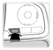
Press the MAIN button on the steering wheel.
