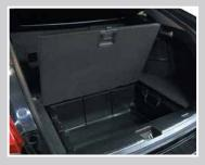
2. **Remove** the hook, and hook it to the cargo side panel to hold the lid in place. **Remove** the cargo box to access the wheel nut wrench in the tool kit.
