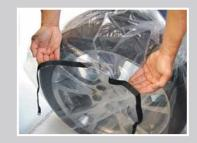
3. **Place** the flat tire in the cargo area. **Thread** the belt through the cargo hook. **Pass** the belt through the ring, and **tighten** the belt to secure the flat tire in place.
