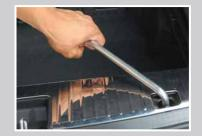
5. Attach the long end of the wrench, and turn it approximately 70 times until you feel resistance and can see the spare tire under the vehicle.
