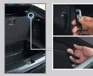
3. **Remove** the plastic cover on the cargo area lining using your key to access the bolt for the spare tire holder.
