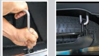
6. **Unhook** the spare tire holder, and **remove** the spare tire.
