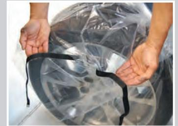
3. **Place** the flat tire in the cargo area. **Thread** the belt through the cargo hook. **Pass** the belt through the ring, and **tighten** the belt to secure the flat tire in place.
