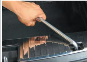
5. **Attach** the long end of the wrench, and **turn** it approximately 70 times. Stop when you feel resistance and can see the spare tire under the vehicle.
