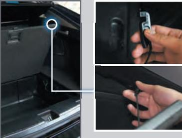
3. **Remove** the plastic cover on the cargo area lining using your key to access the bolt for the spare tire holder.
