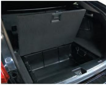
2. **Remove** the hook, and hook it to the cargo side panel to hold the tray in place. **Remove** the utility box to access the wheel nut wrench in the tool kit.
