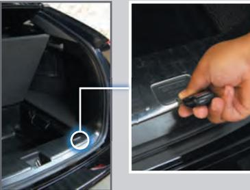
4. **Attach** the short end of the wheel nut wrench to the spare tire holder bolt. **Turn** the wrench counterclockwise until the bolt loosens.
