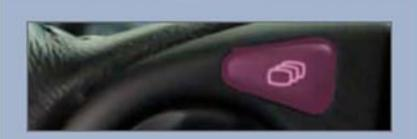
Press the Display button to change the main displays.
