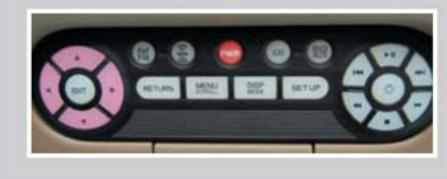
4. The rear control panel can be detached and used as a remote control. **Press** RELEASE to remove it.
