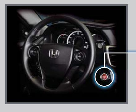
**Press** the ENGINE START/STOP button once (without pressing the brake pedal). **Press** it again for ON mode.
