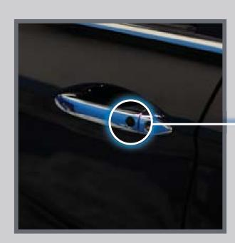
**Press** the door lock button on either front door handle.
