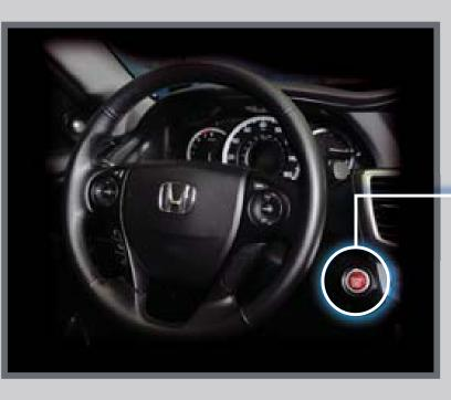
Press and hold the brake pedal\*, then press the ENGINE START/STOP button.
