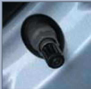
Each tire valve stem contains a TPMS sensor.
