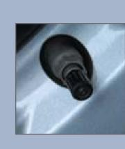
Each tire valve stem contains a TPMS sensor.
