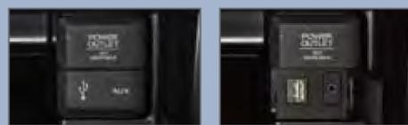
Connect an iPhone or iPod cable or a USB flash drive to the USB port in the front console.
