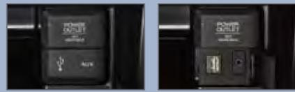
Connect an iPhone or iPod cable or a USB flash drive to the USB port in the front console.
