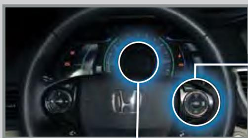
Press the Distance button to shuffle through four ranges.
