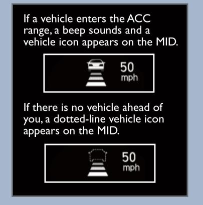
**Note:** The ACC radar sensor in the front grille can detect and monitor the distance of a vehicle up to approximately 100 yards ahead.
