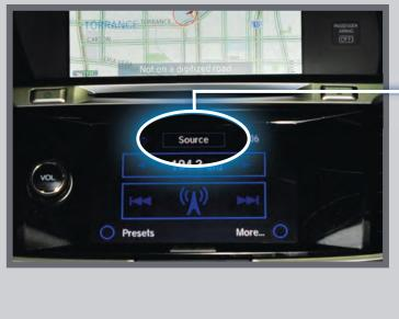
Select the iPod or USB icon from Source. I. Connect the iPod cable or USB flash drive to the USB port in the front console.
