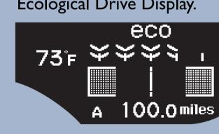
Note: When turned on, performance of the vehicle's engine, transmission, cruise control, and air conditioning system are adjusted to maximize fuel efficiency.
