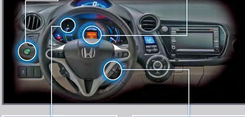
**Note:** When turned on, performance of the vehicle's engine, transmission, cruise control, and air conditioning system are adjusted to maximize fuel efficiency.
