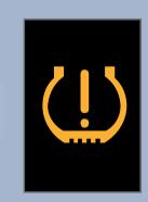
When the tire pressure drops significantly below recommended levels, the low tire pressure indicator comes on and "CHECK TIRE PRESSURE" appears on the MID.
