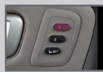
**Note:** Once set, stored positions can be recalled by pressing one of the memory buttons (I or 2) on the door.
