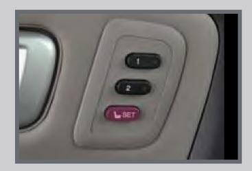
4. Press the memory button corresponding to the remote (I or 2) you are using within 5 seconds. You will hear two beeps.
