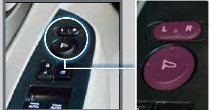
4. Press the memory button corresponding to the remote (1 or 2) you are using within 5 seconds. You will hear two beeps.
