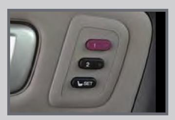
**Note:** Once set, stored positions can be recalled by pressing one of the memory buttons (I or 2) on the door.
