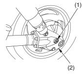
(1) axle shaft(2) final drive gear case
