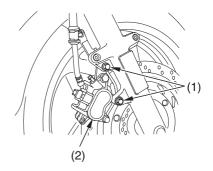
(1) fixing bolts(2) brake caliper assembly
