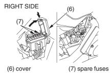
7. To check or replace a circuit fuse, pull the old fuse out of its retaining clips. Look for a burned wire inside the fuse. If the fuse is blown (8), replace it with a spare fuse (7) of the same rating or lower.
