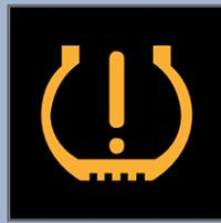
When the tire pressure drops significantly below recommended levels, the low tire pressure indicator comes on.
