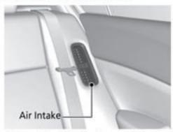
If the air intake is obstructed during vehicle operation, the IMA battery can become too hot. To protect the battery, the system may start limiting IMA battery output power and cause the IMA system and 12 volt battery charging system indicators to come on.
