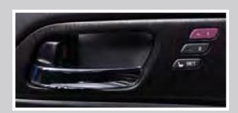
**Note:** Once set, stored positions can be recalled by pressing one of the memory buttons (I or 2) on the door.
