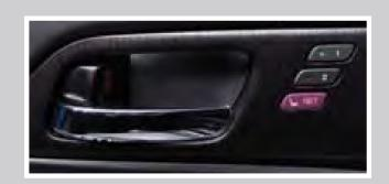
4. Press the memory button corresponding to the remote(I or 2) you are using within 5 seconds. You will hear two beeps.
