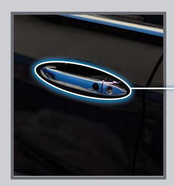
Grab either one of the front door handles when the vehicle is off. Wait until the doors unlock, then pull the handle to open.
