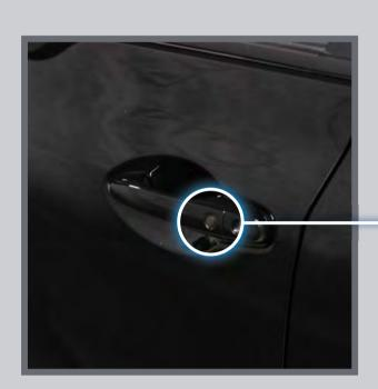
Press the door lock button on either front door handle when the vehicle is off.
