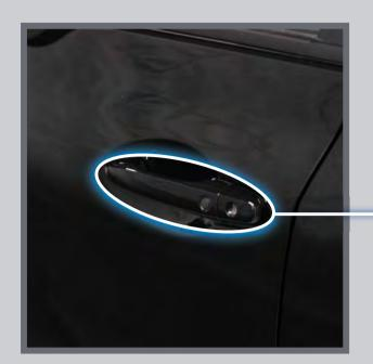
Grab either one of the front door handles when the vehicle is off. Wait until the doors unlock, then pull the handle to open.
