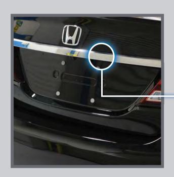
Press the trunk release button under the trunk handle. The vehicle can be on or off.
