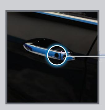
Press the door lock button on either door handle when the vehicle is off.
