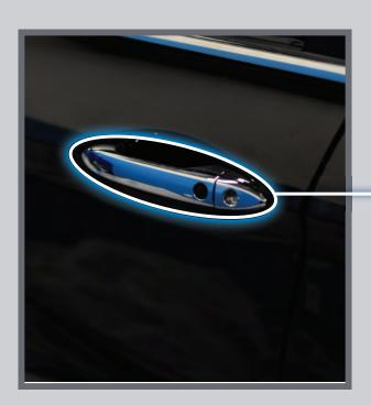
Grab either one of the door handles when the vehicle is off. Wait until the doors unlock, then pull the handle to open.
