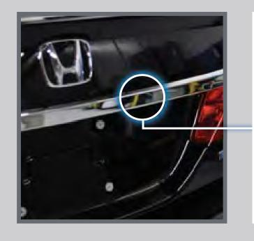
Press the trunk release button under the trunk handle. The vehicle can be on or off.
