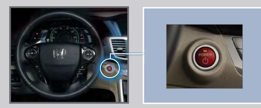
Accessory or On Mode Press POWER once without pressing the brake pedal for Accessory mode. Press it again for ON mode.
