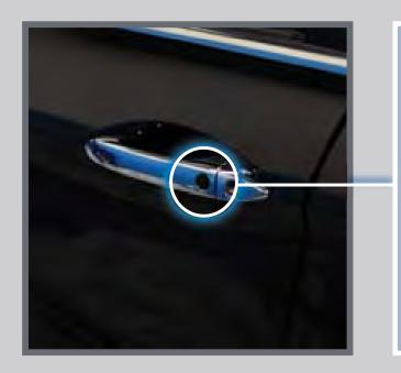
Press the door lock button on either front door handle when the vehicle is off.
