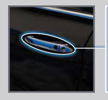
Grab either one of the front door handles when the vehicle is off. Wait until the doors unlock, then pull the handle to open.
