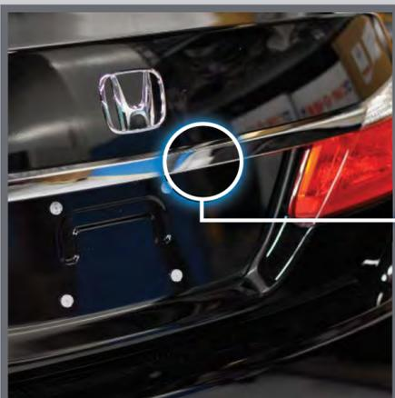
Press the trunk release button under the trunk handle.
