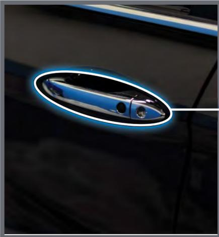
Grab either one of the front door handles when the vehicle is off. Wait until the doors unlock, then pull the handle to open.
