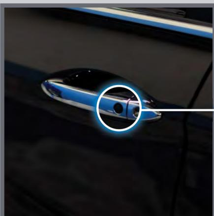
Press the door lock button on either front door handle when the vehicle is off.
