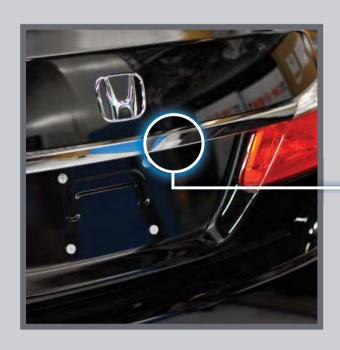
Press the trunk release button under the trunk handle.
