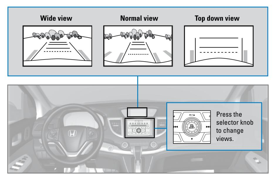
The rear camera view is restricted. You cannot see the corner ends of the bumper or what is underneath the bumper. Its unique lens also makes objects appear closer or farther than they actually are.
