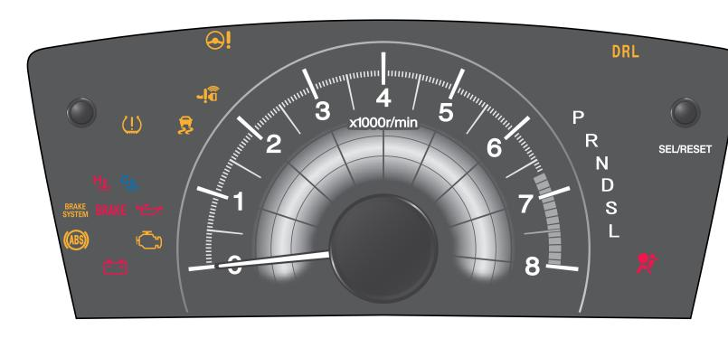
Indicators briefly appear with each engine start and then go out. Red and amber indicators are most critical. Blue and green indicators are used for general information. **Malfunction Indicators**
