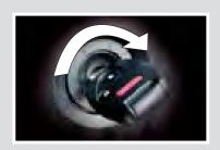
3. Press and hold the unlock side of the master lock switch for about 10 seconds. In that time, you will hear three clicks.
