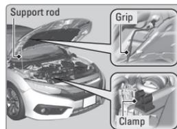
When closing, remove the support rod, and stow it in the clamp, then gently lower the hood. Remove your hand at a height of approximately 12 inches (30 cm) and let the hood close.
