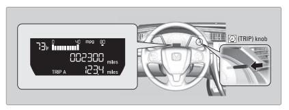
Press the TRIP knob to cycle through the displays shown below.
