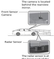
The radar sensor is at the lower part of the front bumper.
