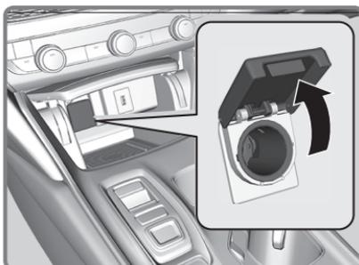
The accessory power socket is designed to supply power for 12-volt DC accessories that are rated 180 watts (15 amps) or less. To prevent battery drain, only use the power socket with the power system on. When both sockets are being used, the combined power rating of the accessories should not exceed 180 watts (15 amps).
