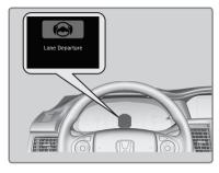
Rapid vibrations on the steering wheel and a warning display alert you that the vehicle is drifting out of a detected lane. The system applies torque to the steering to keep the vehicle between the left and right lane lines. The applied torque becomes stronger as the vehicle gets closer to either of the lane lines. When the vehicle nears a white or yellow line, steering force of the electric power steering will become stronger.
