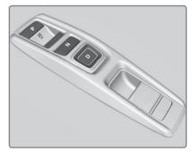
You may occasionally find that it takes longer than usual for the vehicle to start moving when you select Reverse (R). Release and/or depress the brake pedal. This may occur when the High Voltage battery level is extremely low and does not indicate a vehicle malfuction. Always apply the brake pedal before shifting into Park (P) and confirm that the Park (P) is shown on the gear position indicator before releasing the brake.
