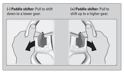
When the transmission is in D: The vehicle goes into sequential shift mode momentarily, and the gear selection indicator comes on. When you start traveling at a constant speed, sequential mode and the gear position indicator automatically go off.
