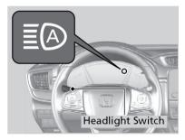
To turn the system on: Pull and hold the headlight lever toward you for about 30 seconds, until the indicator flashes once.
