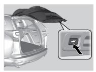
To close the tailgate, press the outer handle again while the tailgate is opening.
